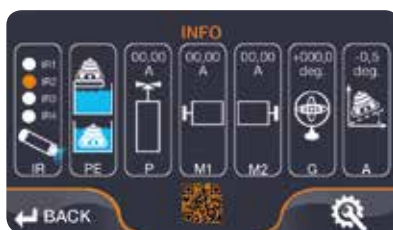
INFO-SETTINGS MENU Robot elements control panel, list of 10 faults, data panel, settings menu
